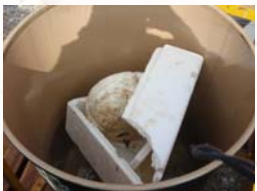
Effective use of foamed polystyrene (Left: Foamed polystyrene, Right: Volume reduction by using SD solvent)
