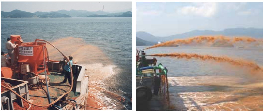
Figure 1.2. Clay dispenser (left) and electrolytic clay dispenser combined with electrolytic seawater generator (right).
