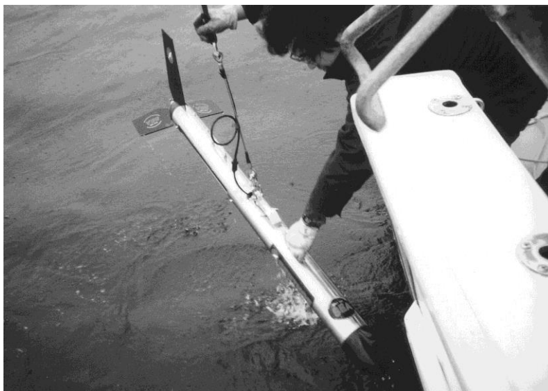
Figure 11. Picture showing towing transducer of side-scan sonar (Komatsu et al. , 2003b)
