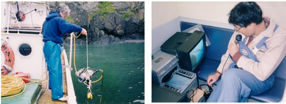
Figure 8. Pictures showing video camera system for sea-truthing in Akkeshi Bay, east Hokkaido. Underwater video camera is lowered from the boat (left picture). An observer monitors bottom features by the display in the cabin (right picture)
