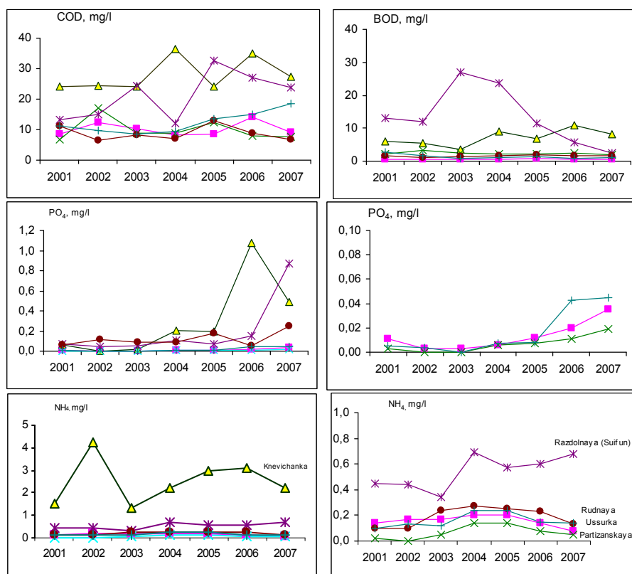
Fig.8.3 Trends of the water quality chemical parameters for some Russian rivers within NOWPAP area
