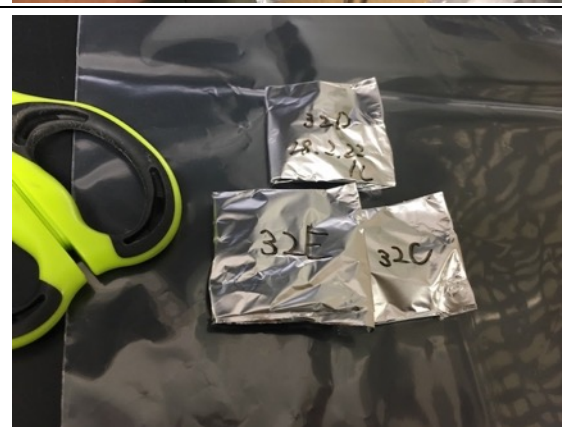
Fig. 3-2-3-6 Write sample information on aluminum foil and store it in a bag, such as a Unipack
