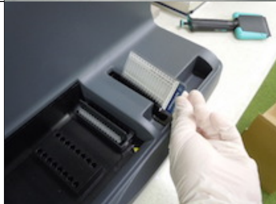
Fig. 5-2-1-3-3 Set ScreenTape and the required number of pipette tips.
