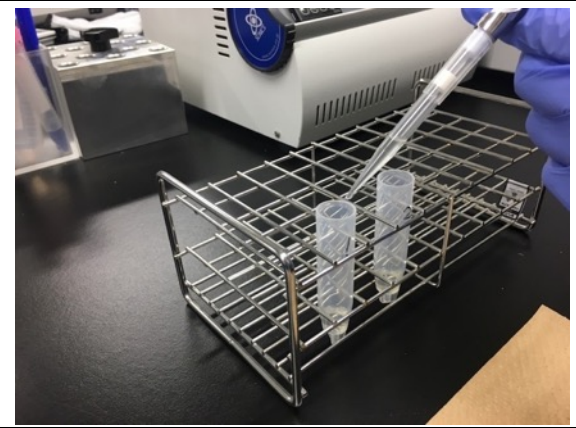
Fig. 4-2-3-2 Remove the upper part of the Salivette tube and add ethanol to the lower part.
