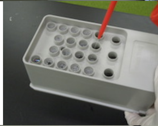
Fig. 5-2-3-1-4 Inject the wash solution into the wash cartridge using the wash bottle.
