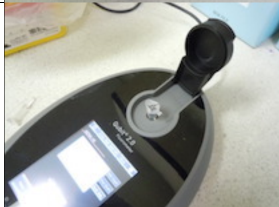
Fig. 5-2-3-8 Measure Standards #1 and #2 in that order according to the instructions from Qubit.
