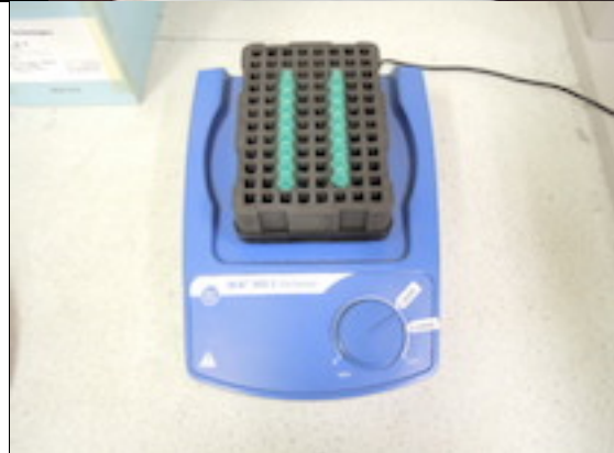
Fig. 5-2-1-3-7 After stirring at 2000 rpm for 1 minute, collect the liquid at the bottom of the tube with a desktop mini centrifuge.
