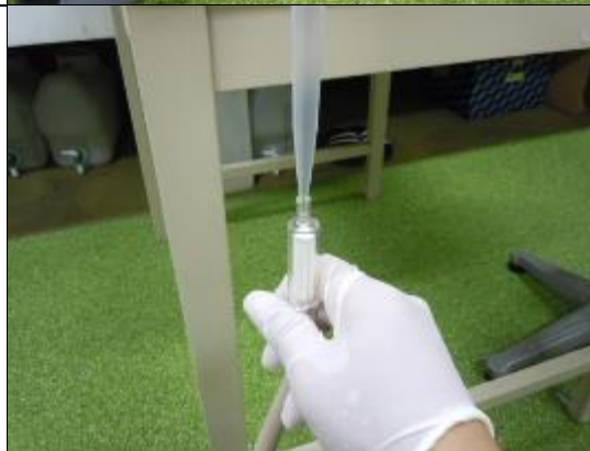
Fig. 3-1-3-8 Insert the end of a 10 mL pipette tip attached to the stopcock of the polyethylene container into the Sterivex filter unit insertion slot.
