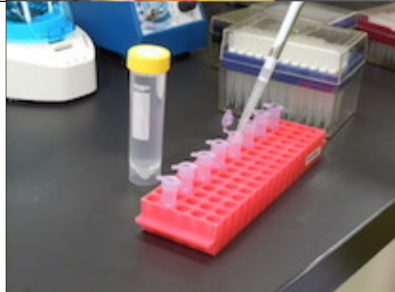
Fig. 5-2-1-2-9 Pipet 700 \mu L of 80% ethanol into the columns.
