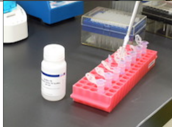
Fig. 5-2-1-2-12 Pipet 90 \mu L of the TE buffer onto the column membrane, let stand for 1 minute, and centrifuge at 20,000 g for 1 minute.
