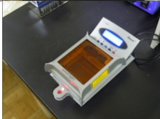
Fig. 5-2-2-4 Set the observation plate unit (unit with an orange filter) on the iBase.
