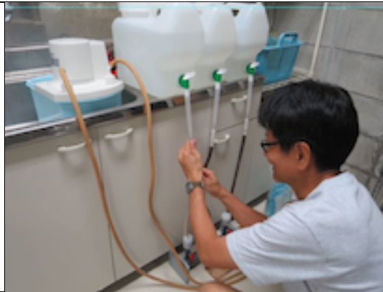
Fig. 3-1-3-9 Mass filtration system using the Sterivex filter units is complete.
