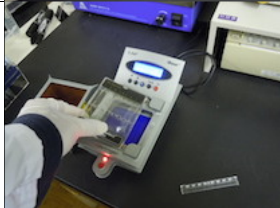
Fig. 5-2-2-2 Insert the cartridge from the right side of the gel into the iBase.
