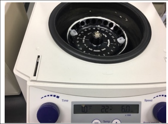
Fig. 4-2-3-6 Pass the solution through the column by centrifuging.
