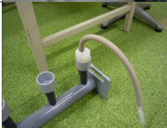
Fig. 3-1-3-7 Attach the above rubber tube to the water absorption hole of the filter holder manifold.
