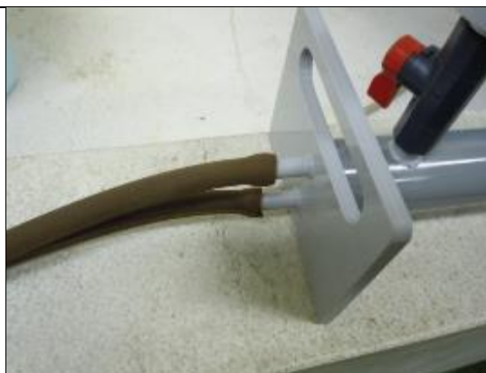
Fig. 3-1-3-5 Connect the outlet port of the filter holder manifold with a rubber tube.
