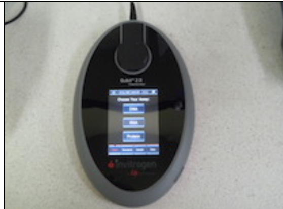
Fig. 5-2-2-3-7 Start the Qubit 2.0 Fluorometer by touching its screen.
