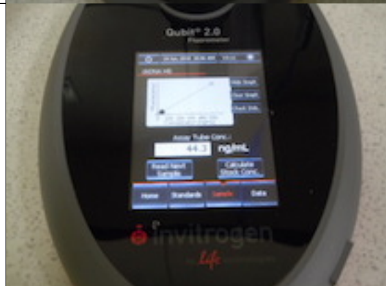
Fig. 5-2-2-3-10 The measured value (ng/mL) of the template diluted 100 times is displayed.
