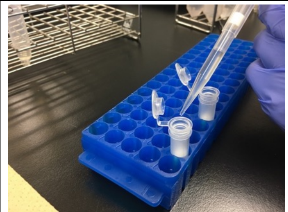
Fig. 4-2-3-5 Transfer the solution in the lower part of the Salivette tube to the DNeasy column.
