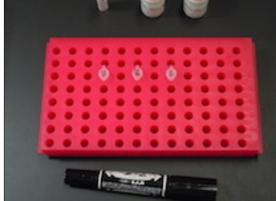
Fig. 5-2-2-3-6 Let stand at room temperature for 2 minutes. If this procedure is omitted, no stable measurements will be obtained.
