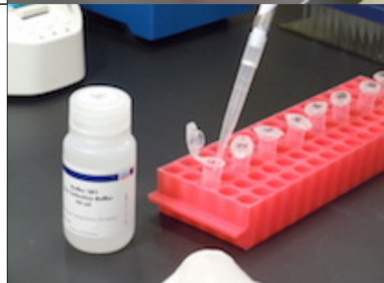
Fig. 5-2-1-2-13 Supplement the collected solution (PCR product obtained after the first purification) with four times the amount of SB1 and pipet the solution.
