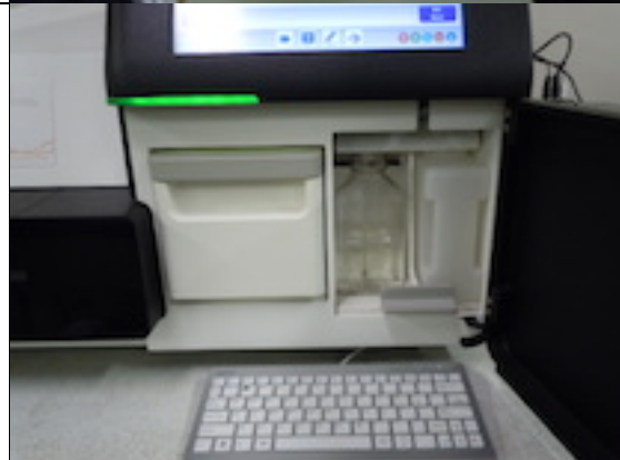
Fig. 5-2-3-1-12 After the bottle is set, pull down the sipper handle. Note that even if you forget to pull down the handle, the run will automatically start.
