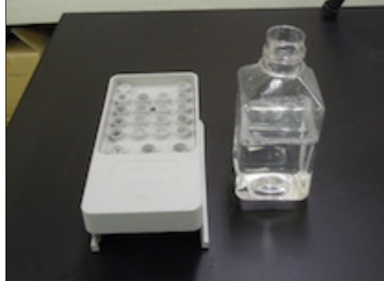
Fig. 5-2-3-1-5 After the wash solution is injected into the cartridge, transfer the remaining wash solution to a wash bottle (about 350 mL).
