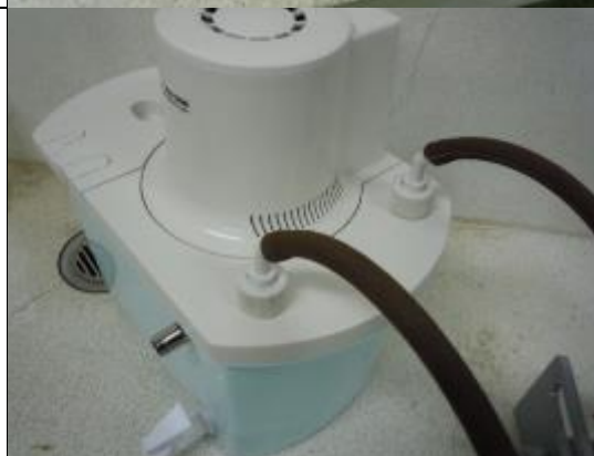
Fig. 3-1-3-6 Connect the rubber tube with the aspirator.
