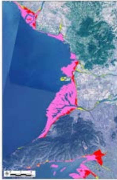
Figure 5. Example of mis-detection of tidal flats in the Ariake Sea.
